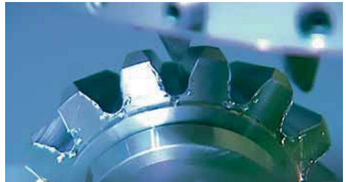
Fig. 5: Bevel gear cut in the Hypoflex® process
