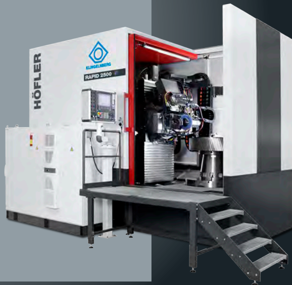
Höfler cylindrical gear grinding machine RAPID 2500 for component diameters of up to 2,500 mm
